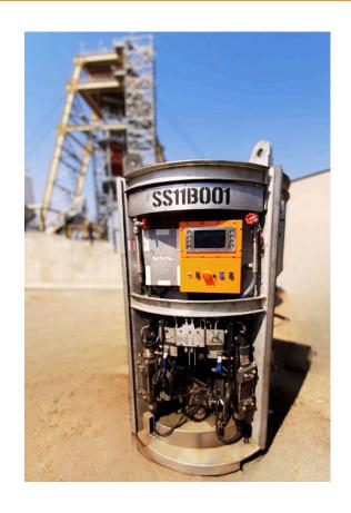
The system is designed with a spectrum of sensors to monitor all aspects of pumping operations. This operator practices together with safety critical sensors, hydraulic supply and the charge mass per hole. This allows for the utmost in safety, product consistency and machine availability in UN Class 5.1 loading operations.
