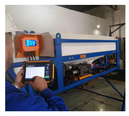
Through the implementation of SMARTFLOW<sup>TM</sup> pump technology, optimal safety, product consistency and machine availability can be improved throughout loading operations. SMARTFLOW<sup>TM</sup> pumps are designed as standalone explosive manufacturing systems that deliver selectable predetermined ratios of emulsion, sensitizer and hose lube during loading operations for improved consistency and reduced downtime.
