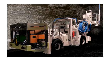
Flexible control of the SMART**RING™** Pumping System is achieved through the BLAST**TRACK™** control system. The safety and control system uses a range of safety and performance sensors throughout the pumping and loading system to facilitate optimal product delivery, hose retraction, reel and boom control. The pumping systems can controlled from the remote control panels in a loading basket or standing away from the system in a designated safety area.
