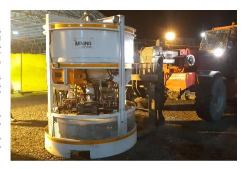
The SMARTFLOW<sup>TM</sup> emulsion pumps can be controlled through a handheld remote to the BLASTTRACKTM Controller. This allows for easy operating where communication is difficult. The shaft sinking pod has been designed on a plug and play basis, meaning should a breakdown occur, the part can simply be swopped within a few minutes to restart the charging process on that pump, resulting in one of the most efficient shaft sinking pods created.
