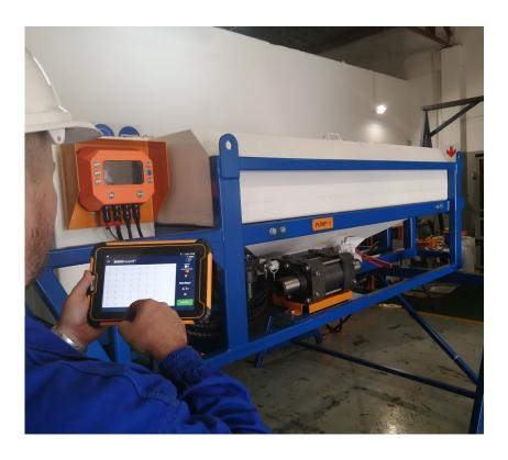
Through the implementation of SMARTFLOW<sup>TM</sup> pump technology, optimal safety, product consistency and machine availability can be achieved throughout loading operations. SMARTFLOW<sup>TM</sup> pumps are designed as standalone explosive manufacturing systems that deliver selectable predetermined ratios of emulsion, sensitizer and hose lube during loading operations for improved consistency and reduced downtime.
